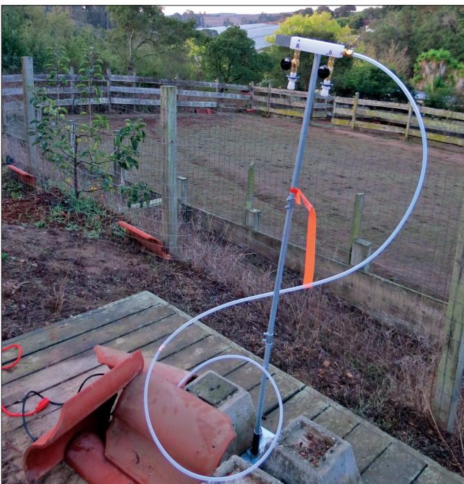
Drift Catcher equipment for monitoring the fumigant chloropicrin in Justin's backyard where his children play. The tarps of the fumigated strawberry field are visible in the distance. He found concentrations of chloropicrin that pose an increased risk of cancer.
